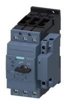
Circuit breaker size S2 for motor protection, CLASS 10 with overload relay function A-release 35...45 A N-release 650 A Standard switching capacity
