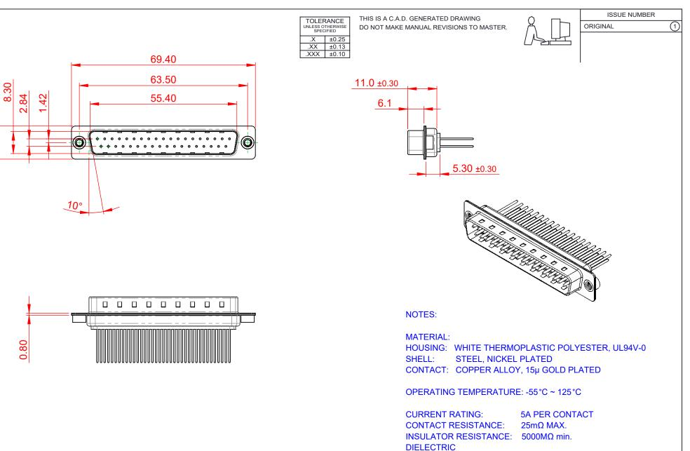
WITHSTANDING VOLTAGE: 1000V AC rms
