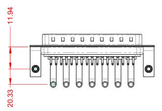
30A (CURRENT) **POWER/CO-AX CONTACT RATING:** (IF PRESENT) SIGNAL CONTACT CURRENT RATING: 5A PER CONTACT SIGNAL CONTACT RESISTANCE:  $10m\Omega$  MAX. **INSULATOR RESISTANCE:** 5000MΩ min.
