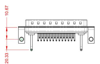
**OPERATING TEMPERATURE:** -55°C ~ 125°C 10A (CURRENT) POWER/CO-AX CONTACT RATING: (IF PRESENT) SIGNAL CONTACT CURRENT RATING: 5A PER CONTACT SIGNAL CONTACT RESISTANCE:  $10m\Omega$  MAX. **INSULATOR RESISTANCE:** 5000MΩ min. DIELECTRIC
