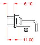
THERMOPLASTIC POLYESTER, UL94V-0 STEEL, NICKEL PLATED COPPER ALLOY, 30µ" GOLD PLATED
