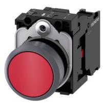
Pushbutton, 22 mm, round, plastic with metal front ring, red, pushbutton, flat, momentary contact type, with holder, 1 NC, screw terminal, with laser labeling, upper case
