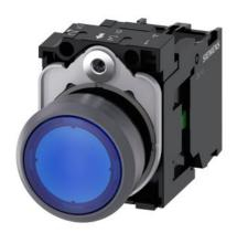
Illuminated pushbutton, 22 mm, round, plastic with metal front ring, blue, pushbutton, flat, momentary contact type, with holder, 1NO, LED module with integrated LED 110 V AC, screw terminal, with laser labeling, symbol number according to, ISO 7000 or IEC 60417
