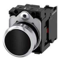
Pushbutton, 22 mm, round, metal, shiny, black, pushbutton, flat, momentary contact type, with holder, 1 NC, screw terminal, with laser labeling, lower case
