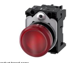
Indicator lights, 22 mm, round, metal, shiny, red, lens, smooth, with holder, LED module with integrated LED 110 V AC, screw terminal, with laser labeling, inscription or symbol Customer-specific selection with SIRIUS ACT configurator (CIN)
