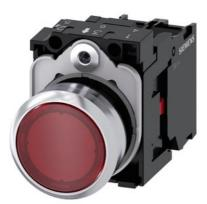
Illuminated pushbutton, 22 mm, round, metal, shiny, red, pushbutton, flat, momentary contact type, with holder, 1NC, LED module with integrated LED 230 V AC, screw terminal, with laser labeling, upper case and lower case, Always upper case at the beginning of the word
