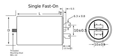
General Information Series C27 Dielectric Film/Foil Polypropylene Style Plastic Case and Cover, Ultra Sonically Welded Description Ultra Sonically Welded Seal, Safety Class PO, Features UL 94 V0 Disk **RoHS** Yes Lead Fast On (1+1) UL, VDE, UL (Construction Only), UL\_94 VO Qualifications Disk AEC-Q200 No Component 52 g Weight
