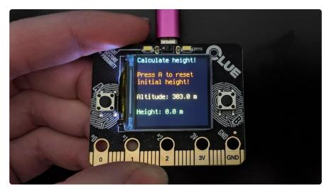
The Adafruit CLUE has a barometric pressure sensor that uses the pressure readings to calculate altitude. For more information on how this works, check out Wikipedia ().
