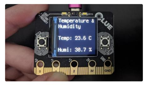
The Adafruit CLUE has a temperature and humidity sensor that reads the temperature in degrees Celsius and the relative humidity in percent. To learn more about relative humidity, check Wikipedia ().
