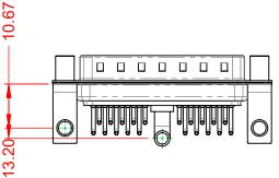
40A (CURRENT) POWER/CO-AX CONTACT RATING: (IF PRESENT) SIGNAL CONTACT CURRENT RATING: 5A PER CONTACT SIGNAL CONTACT RESISTANCE:  $10m\Omega$  MAX. **INSULATOR RESISTANCE:**
