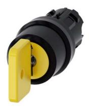
Key-operated switch O.M.R, 22 mm, round, plastic, lock number 73033, yellow, with 2 keys, 3 switch positions I-O-II, latching, actuating angle 2x45°, 10:30h/12h/13:30h, Key removal I+O+II, with laser labeling, lower case
