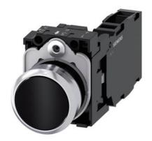
Pushbutton, 22 mm, round, metal, shiny, black, pushbutton, flat, momentary contact type, 1 NO+1 NC, screw terminal, with laser labeling, symbol number according to, ISO 7000 or IEC 60417
