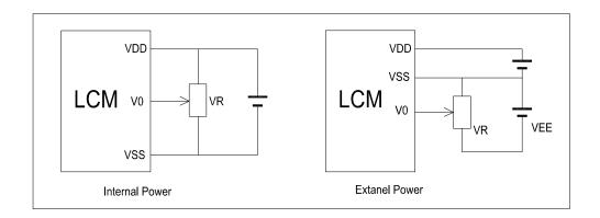
$V_{DD\sim}V_0$ : LCD Driving voltage VR:  $10k\sim20k$
