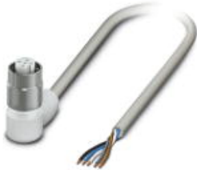
Sensor/Actuator cable, 5-position, PP-EPDM halogen-free, Gray RAL 7035, Free cable end, on Socket angled M12, A-coded, Cable length: 5 m, Hygienic design, With high-grade steel knurl
