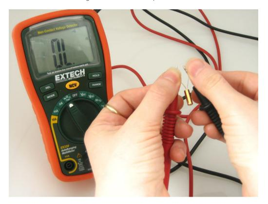
When pointing down, the switch is Open Loop (no continuity).
