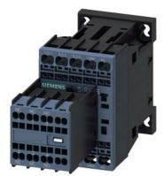
power contactor, AC-3 12 A, 5.5 kW / 400 V 2 NO + 2 NC, 230 V AC 50 / 60 Hz, 3-pole Size S00, Spring-type terminal Removable auxiliary switch
