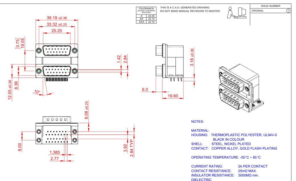
WITHSTANDING VOLTAGE: 1000V AC rms
