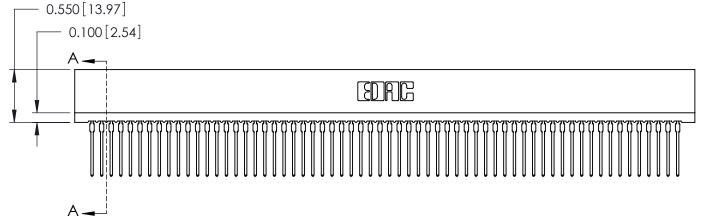
725 Series Ultra-Mate Card Edge Connector - Press Fit Part Number: 725-124-540-201
