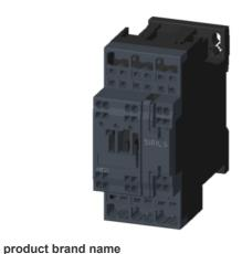
power contactor, AC-3 25 A, 11 kW / 400 V 1 NO + 1 NC, 110 V AC, 50 Hz, 120 V, 60 Hz, 3-pole, Size S0, Spring-type terminal Multi-unit packaging = 18 units
