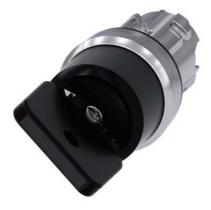
Key-operated switch O.M.R, 22 mm, round, metal, shiny, lock number 73034, black, with 2 keys, 2 switch positions O<I, momentary contact type, Actuating angle 45°, 10:30h/12h, key removal O, with laser labeling, inscription or symbol Customer-specific selection with SIRIUS ACT configurator (CIN)
