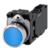
Pushbutton, 22 mm, round, metal, shiny, blue, pushbutton, flat, momentary contact type, 1 NO+1 NC, screw terminal, with laser labeling, upper case
