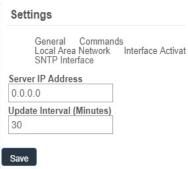
SNTP Interface – SNTP is a synchronized computer clock on a network. An SNTP server can be set up on the same LAN as the gateway, such as on a router or a Linux computer. The gateway should be configured to retrieve time from only trusted servers, such as ones maintained by your ISP. Incorrect time can affect the delivery of sensor traffic
