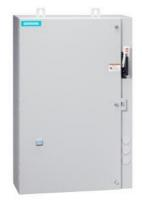
Non-reversing motor starter, Size 2, Three phase full voltage, Solid-state overload relay, OLR amp range 13-52A, Combination type, 60A non-fusible disconnect, Encl NEMA type 4X 304 S-Steel, Water/dust tight noncorrosive, Extra-wide enclosure
