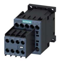
Power contactor, AC-3 16 A, 7.5 kW / 400 V 24 V DC, with diode integrated 3-pole, Size S00 screw terminals 1 NO integrated 2 NO + 2 NC plugged on
