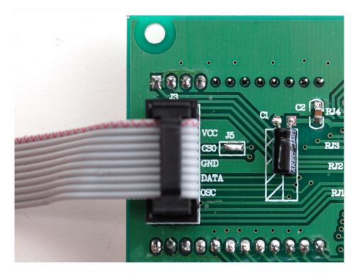
Begin by plugging in a 2x5 pin IDC cable into the top left socket:
