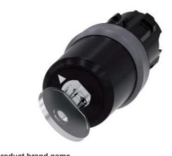
Key-operated switch BKS, 22 mm, round, plastic with metal front ring, Lock No. E2 (VW), without key, 2 switch positions O-I, latching, actuating angle 90°, 10:30h/13:30h, key removal O+I, with laser labeling, inscription or symbol Customer-specific selection with SIRIUS ACT configurator (CIN)
