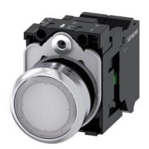
Illuminated pushbutton, 22 mm, round, metal, shiny, white, pushbutton, flat, momentary contact type, with holder, 1NO, LED module with integrated LED 110 V AC, spring-type terminal, with laser labeling, upper case
