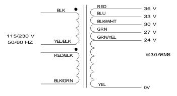
**Technical note:** Primary windings are designed to be connected in series or parallel.
