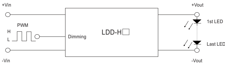
Fig-1 12VDC input, 1~3 LEDs (Vf=3V)
