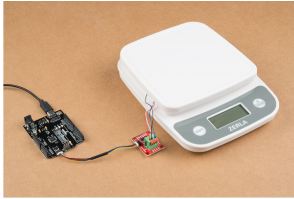
Four arms in correct position with four wires connected to BlackBoard
