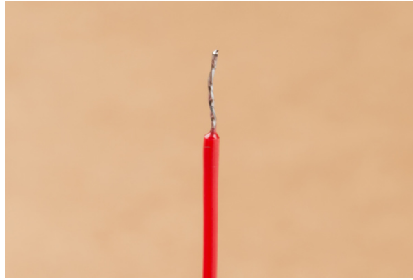
Twisted stranded wire tinned with solder
