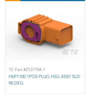
Housing for Male Terminals, 1 Position, Sealable, Orange, Cable Mount (Free-Hanging), -40 – 257 °F [-40 – 125 °C], Key B
