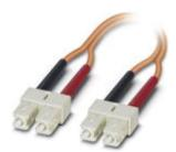
Assembled FO cable, zip cord cable, multi-mode fiberglass 62.5/125 µm, OM1, connector: SC duplex/SC duplex, degree of protection: IP20, for installation in cable ducts or control cabinets
