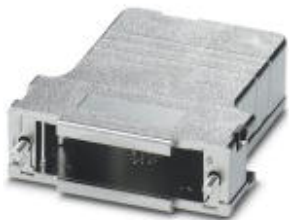
D-SUB sleeve housings, degree of protection: IP20, material: ABS, metal-plated, cable outlet: angled, size of housing: 3, color: Bare metallic
