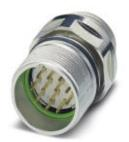
Device connector for front wall, straight, shielded: yes, for standard and SPEEDCON interlock, M23, No. of pos.: 17, type of contact: Pin, Crimp connection, Axial seal, Central fastening M20 x 1.5, can be positioned via a locking nut
