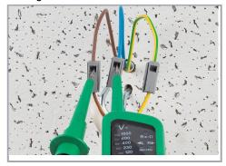
Testing via separate test ports.
