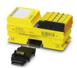
Safety-related digital output module, IP20 protection, for the SafetyBridge system. The module has four safe digital outputs with two-channel occupancy or 8 safe digital outputs with single-channel occupancy
