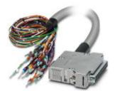
Assembled shielded round cable; connection 1: Single wires (37-position) (The wires are marked and fitted with ferrules.); connection 2: D-SUB socket strip (1x 37-position); cable length: 1 m
