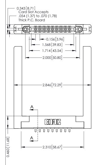
SECTION A-A 0.295[7.49] Card Slot 0.090[2.29] Point of Contact 305 ENG MASTER 305 / 315 / 355 Card Edge Connector DATE: SEPT. 21/09 J.LEE Part Number: 355-018-521-258
