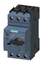
Special type Circuit breaker size S00 for motor protection, CLASS 10 Arelease 9...12 A N-release 163 A screw terminal Standard switching capacity Ambient temperature -50  $^{\circ}\text{C}$  500 switching cycles
