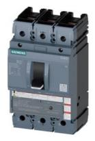
circuit breaker 3VA5 UL frame 250 breaking capacity class M 35kA @ 480 V 3-pole, line protection TM210, FTFM, In=110A overload protection Ir=110A fixed short-circuit protection Ii=10 x In UL489 SB (naval), 50 deg. cel. nut keeper kit on both sides
