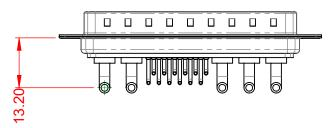
20A (CURRENT) POWER/CO-AX CONTACT RATING: (IF PRESENT) SIGNAL CONTACT CURRENT RATING: 5A PER CONTACT SIGNAL CONTACT RESISTANCE:  $10m\Omega$  MAX. 5000MΩ min. **INSULATOR RESISTANCE:** DIELECTRIC
