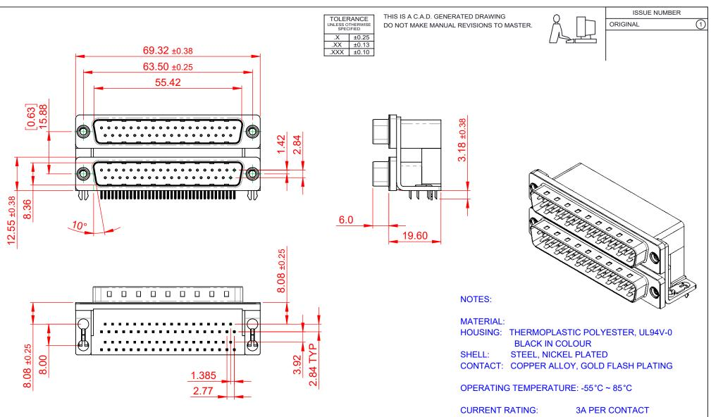
CORRENT RATING: 3A PER CONTA CONTACT RESISTANCE: 25mΩ MAX. INSULATOR RESISTANCE: 5000MΩ min. DIELECTRIC WITHSTANDING VOLTAGE: 1000V AC rms
