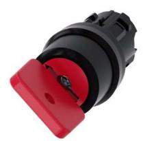
Key-operated switch O.M.R, 22 mm, round, plastic, lock number 73037, red, with 2 keys, 2 switch positions O-I, latching, actuating angle 90°, 10:30h/13:30h, key removal O+I, with laser labeling, upper case and lower case, always upper case at beginning of line
