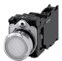
Illuminated pushbutton, 22 mm, round, metal, shiny, white, pushbutton, flat, momentary contact type, with holder, 1 NO+1 NC, LED module with integrated LED 24 V AC/DC, spring-type terminal, with laser labeling, upper case and lower case, always upper case at beginning of line
