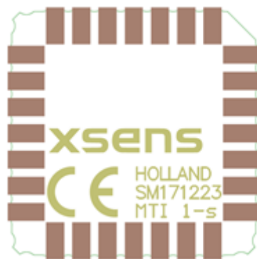
Location PCB number on MTi 1-series module (bottom view)
