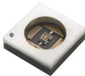
QLUV07N2EM 3535 10mW UVC LED
