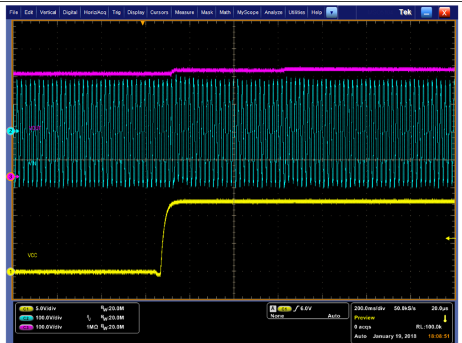
Figure 12. 265 VAC Start-up No Load
